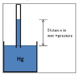
A manometer is a device for measuring the relative pressure inside of a container:
